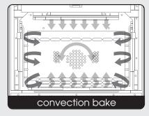
meats on the outside and retaining more juices and natural flavor on the inside with less shrinkage. This even circulation of air equalizes the temperature throughout the oven cavity and eliminates the hot and cold spots found in conventional ovens.
